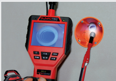
Pipe inspection as of pipe - Ø 20 mm
