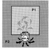
Temperature-related pressure differences between the inside of the enclosure (P1) and the surrounding atmosphere (P2) are balanced by the breather. The amount of condensation forming in the enclosure is thus kept to a minimum.
