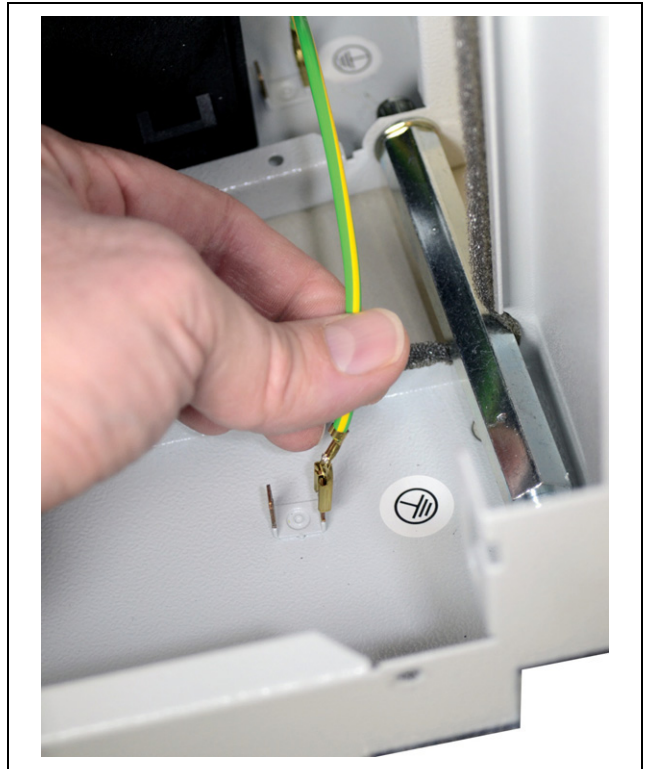
Fig. 26: Disconnect the ground cable between the cover and chassis
