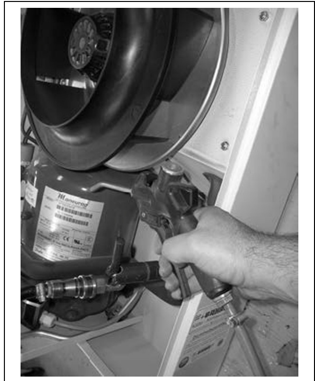
Fig. 31: Clean out the heat exchanger coil and compressor chamber using compressed air
