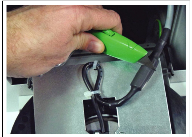
Fig. 27: Cut heat shrink tubing around circumference of connector
