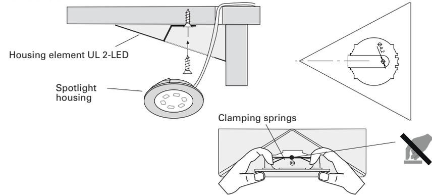
Remove protection foil from housingsurface UL 2-LED before mounting. Place housingelement UL 2-LED in the required position. Fix housingelement with screw through the lug hole. Fit LED-spotlight in place (clamping springs parallel to the wall).
