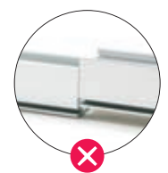
parallel horizontal misalignment
