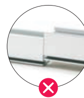
parallel vertical misalignment
