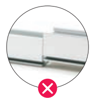
parallel horizontal misalignment
