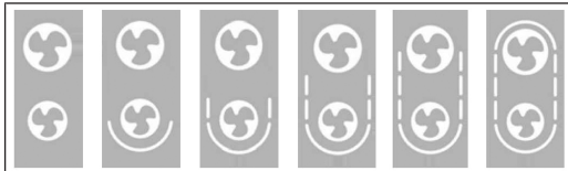
Ventilation level indication by number of symbol bars: 0 (off) to ventilation level 5
