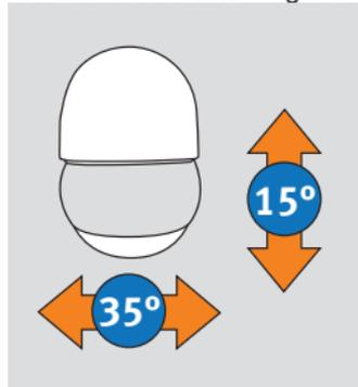
Horizontal turning of the sensor head approx.  $\pm 35^\circ$  (see illustration)
