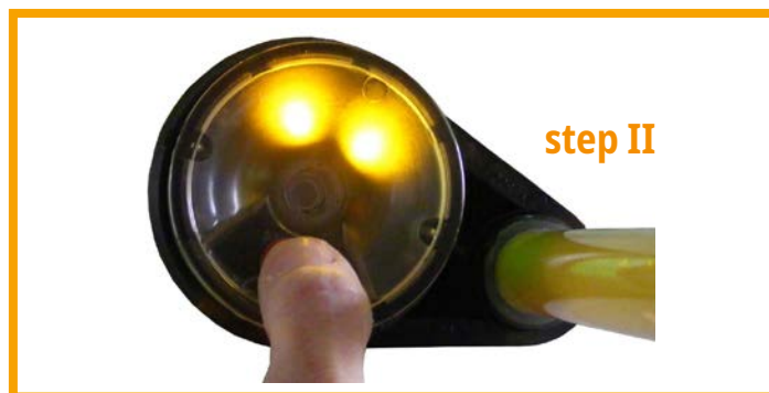
Fig. 6 Switching the phase comparator on/step II
