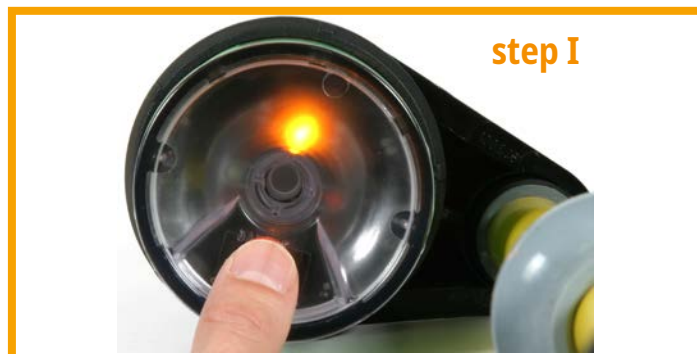
Fig. 5 Switching the phase comparator on/step I
