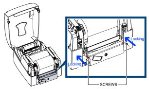
**STEP-04** Pass the labels through the guides and close the printing mechanism.
