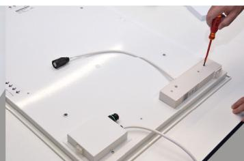
3. Insert the plug connection into the controller and screw together.
