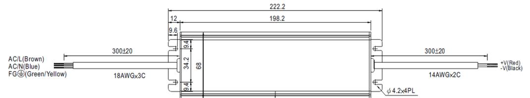
Do not install other power cables along this LED driver to avoid high frequency interference.
