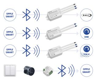
Easily integrate any existing luminaire, be it 1-10V, Triac or DALI2, into the Smart System with our converters.
