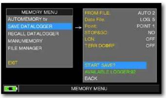
Set the parameters required. Touch "START SAVE" to create a new log file.
