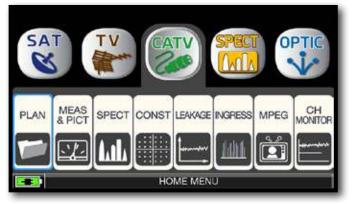
Touch "CATV" and then "PLAN" or use the encoder to access at the CATV canalizations list.
