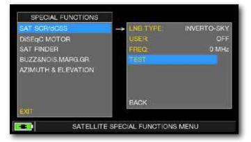
Or touch "TEST", in Spectrum mode, to perform a verify of the 4 exit frequencies (user 1-4) from LNB/multiswitch.
