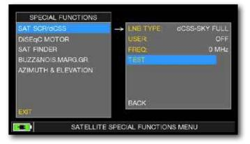
Or touch "TEST", in Spectrum mode, to perform a verify of the 12 exit frequencies (user 5-16) from LNB/multiswitch.
