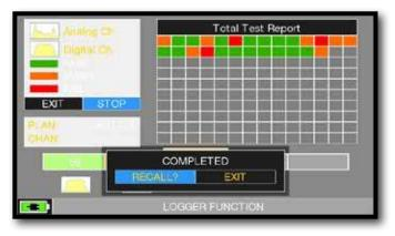
Touch "RECALL" to recall the Logger or "EXIT" to exit.
