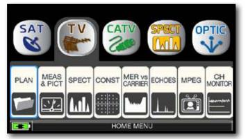
Touch "TV" and then "PLAN" or use the encoder to access at the TV canalizations list.
