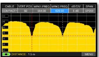
In the DISTANCE window, read the cable's mismatching value: example 1.5 m.
