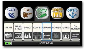
Touch "CATV" and then "LEAKAGE" or use the encoder.
