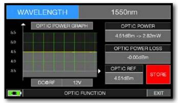
Touch "STORE" and memorizes the measured optical power value (Optic Ref.): for Example 4,51 dBm.
