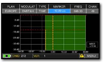
MicroEchoes visualization, touch the Marker and rotate the encoder to select the ECHOES.
