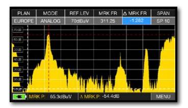
C/N measurement mode "OUTSIDE THE BAND": The signal/noise ratio is measured between the signal level of the video carrier (signal/carrier, red marker) and the noise level estimated in the guard band (-1.282 MHz from the video carrier, white marker).
