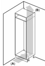
A: Air inlet  $\geq 200$  cm<sup>2</sup>; Ventilation options
