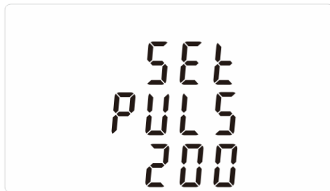
(It shows pulse width of 200ms)
